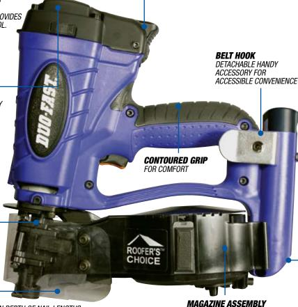
TOOL SPECIFICATIONS **MODEL NUMBER:** DFCR175C PART NUMBER: 904600 **WEIGHT:** 6.8 LBS LENGTH: 11.5" **CYCLE RATE:** 2-3 NAILS P/SEC. BATTERY: 2,200 NAILS P/CHG. **FASTENER SPECIFICATIONS** SHANK DIAMETERS: .120 NAIL LENGTH: 7/8"-1-3/4" ROOFER'S CHOICE FOR MAX. **FASTENER TYPE:** PERFORMANCE, USES ANY
